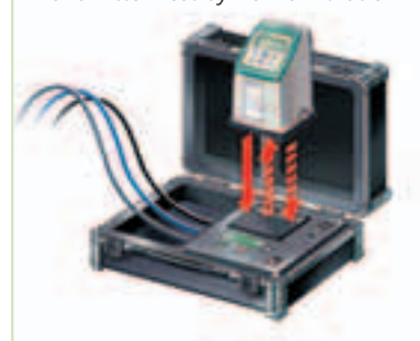
Transmitter Test by flow simulation
